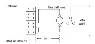
NOTE: The wire length from indoor unit to the Relay must be within 2,0m. Pulse signal changeable to static with JP cutting. (Refer to JP001)
