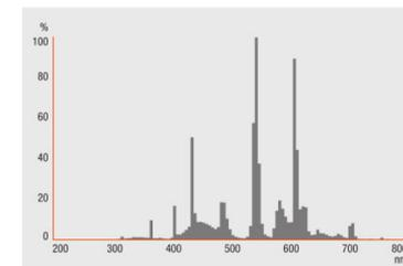
HO 24 W/827, HO 24 W/830, HO 24 W/840, HO 24 W/865, HO 39 W/827, HO 39 W/830, HO 39 W/840, HO 39 W/865, HO 49 W/827, HO 49 W/830, HO 49 W/840, HO 49 W/865, HO 54 W/827, HO 54 W/830, HO 54 W/835, HO 54 W/840, HO 54 W/865, HO 54 W/880, HO 80 W/827, HO 80 W/830, HO 80 W/840, HO 80 W/865
